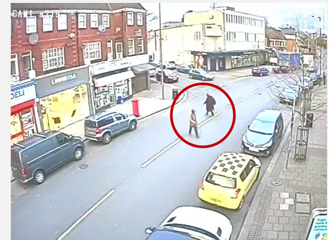
Due to poor crossing provision, pedestrians cross ad-hoc increasing risk of collisions
