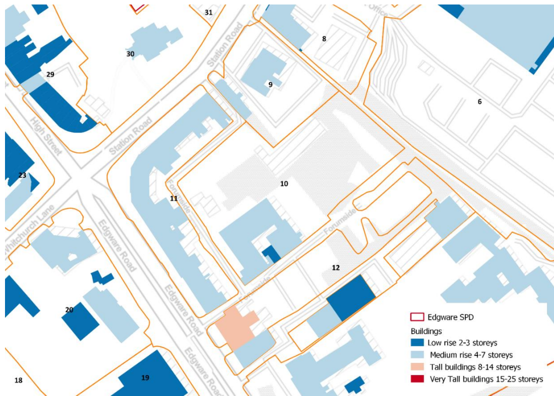
Figure 26 Existing building heights (note the plan is derived from an analysis of heights in metres translated to storeys and therefore the number of storeys is indicative)
