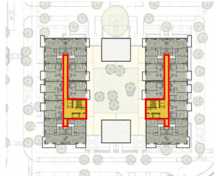
Figure 35: Typical podium block upper floor access
